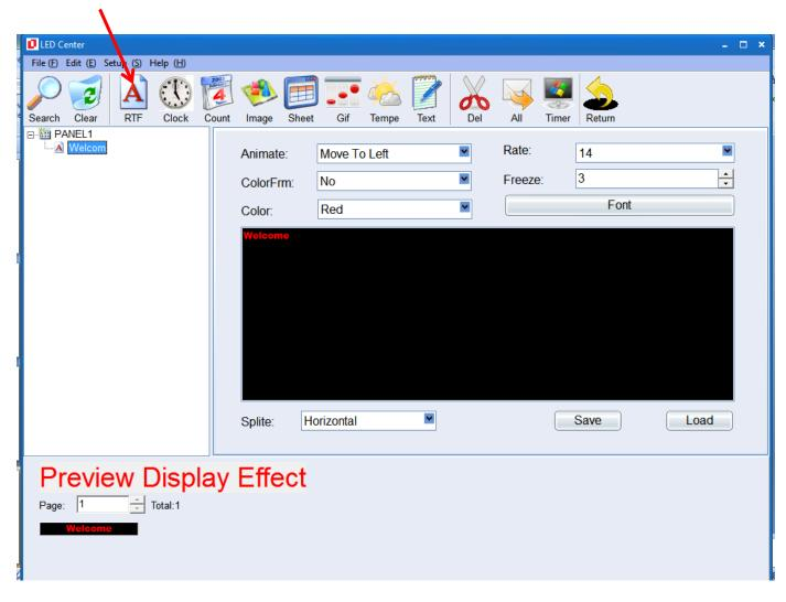
Step 6. After you finish the message set up, you can send the message to LED SCREEN directly by clicking All (LED Screen should be connected to computer) or you can save the setup program by clicking file/export SD/USB card format. Take the USB and insert in the USB connect in the LED screen .
